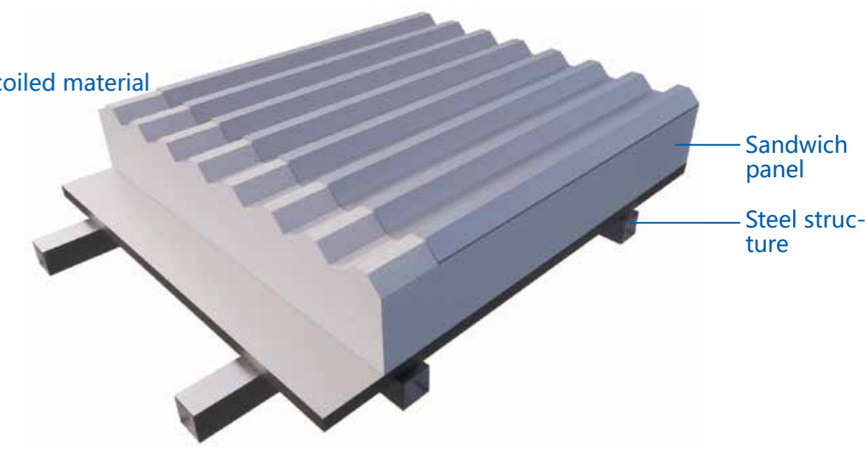
Roof construction drawing II (sandwich panel)
